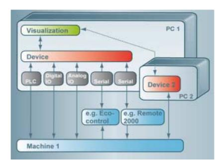
Communication between the two modules usually takes place within the PC. However, it is also possible to connect additional drivers via network links.
